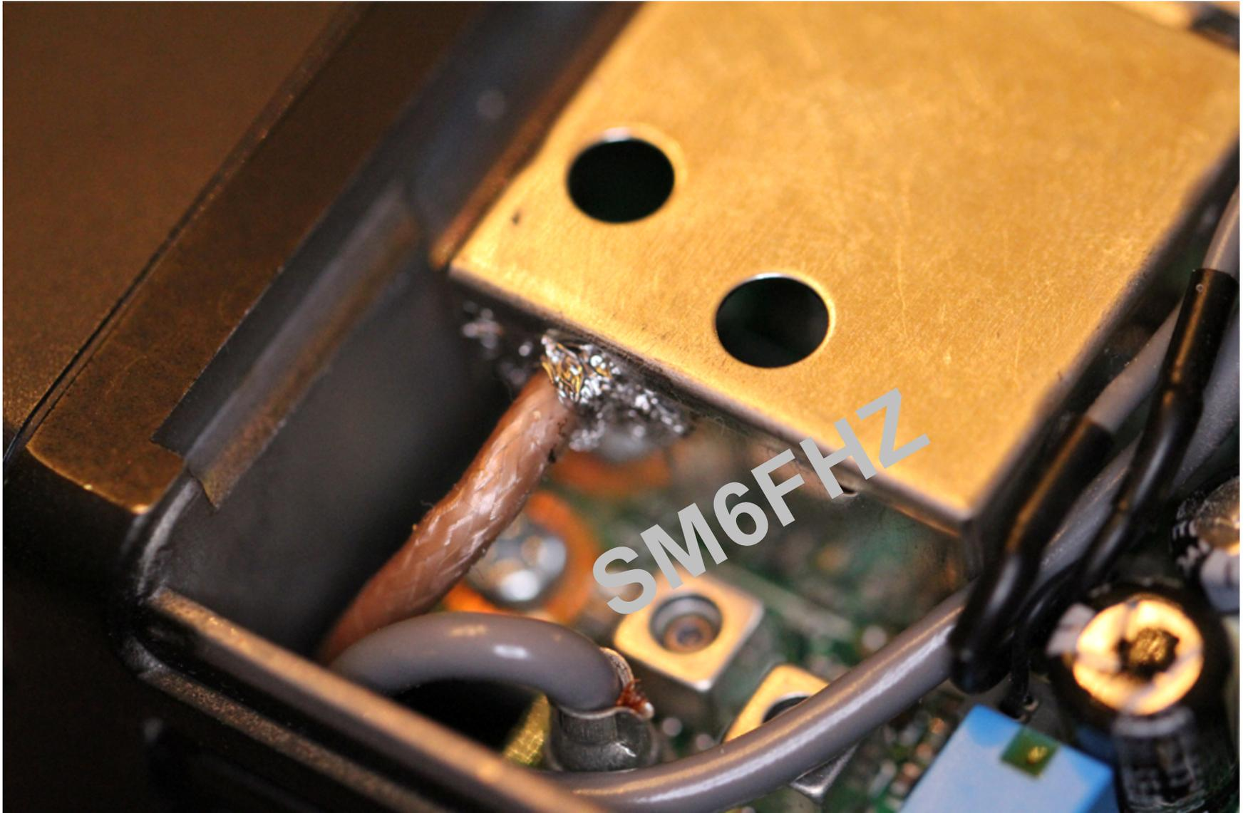
Wind a 6 turn coil that fits on the L601 coil in the oscillator box.
